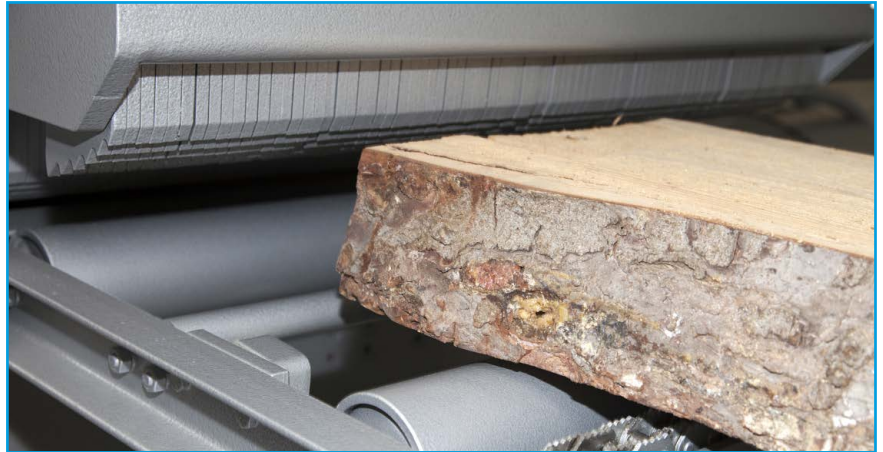
Fig. 9: Anti-kickback device for increased safety
