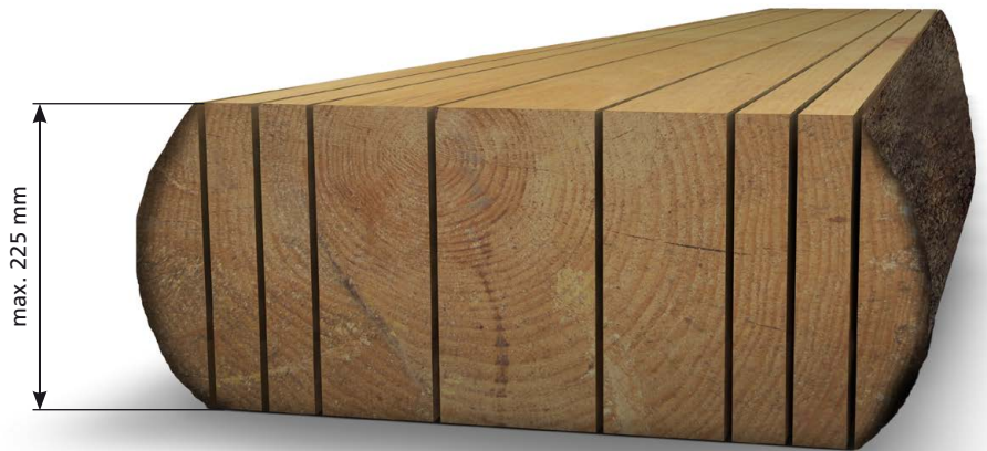
Fig. 6: Possible ripping pattern
