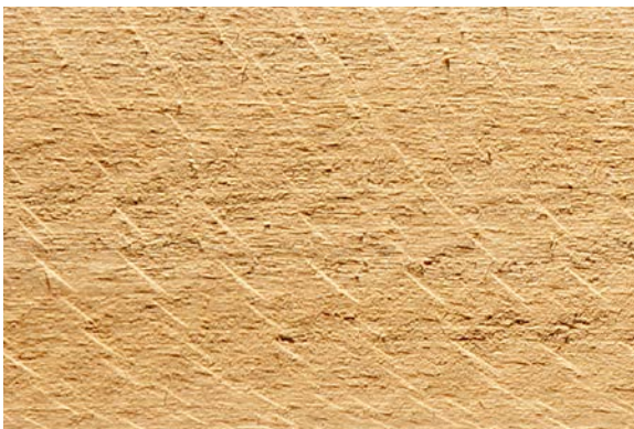
Fig. 4: Cutting quality achieved on a conventional rip saw.
