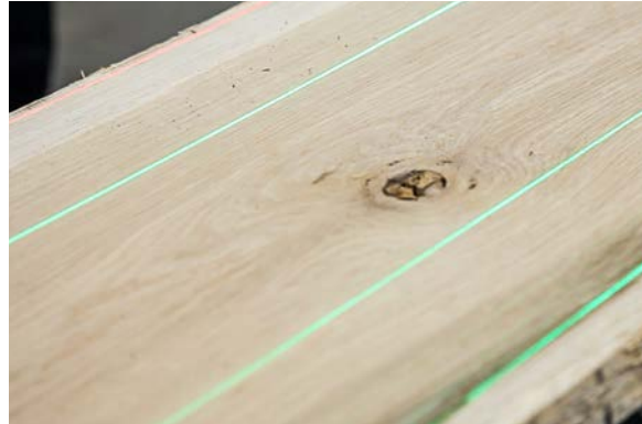
Fig. 9: Line laser for an easy workpiece alignment and optimum workpiece segmentation.
