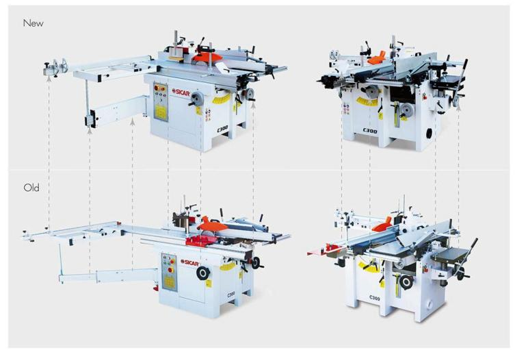
**The C300 Combined Machine** has been specifically designed be an industrial standard machine, but at a size intended for the factory and small professional workshop. This industrially rated machine features a table saw and sliding table, planer, thicknesser and spindle moulder unit. The cast iron construction, accurate cross cut fence and superb build quality put this machine in a class of its own.
