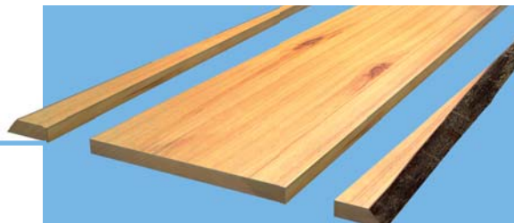
Fig. 24: Separation of boards and edgings by the offcut separator
