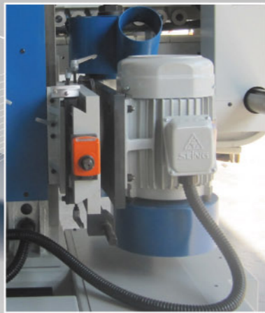
Moulding unit (R) 5HP (option 7.5HP) Spindle speed: 6000 RPM Spindle size: Ø40 MM x 120 MM Space required: 450 MM
