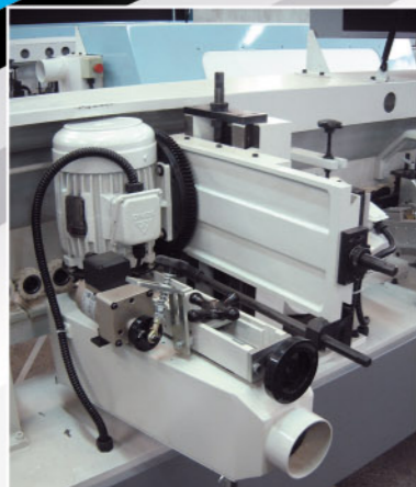
Roller Type Belt sanding unit Motor: 2 HP Sanding belt size: 4" x 42" With Vibration motor Rubber roller: Diameter 7" x Length 4" Space required: 300 MM
