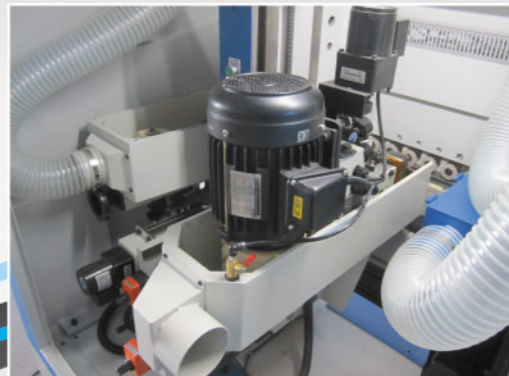
Belt sanding unit Motor: 2 HP Sanding belt size: 4" x 60" Vibration power: 25w x 1/36 Space required: 300 MM
