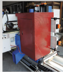
安全防护网 Safety net Prevent wood dust from spraying
