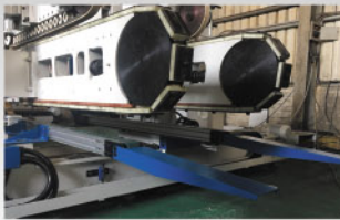
回料装置 Feedback conveyor Transfer the working piece back through the conveyor belt.
