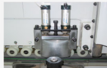
Moulding unit with pneumatic top pressure pad+bottom support (Chrom plated)
