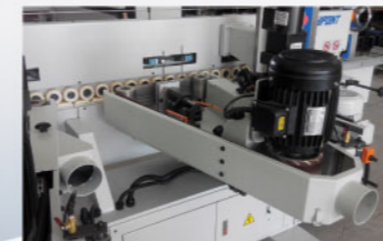
Profile belt sanding Motor : 2HP Sanding belt size : 4"x 98"/ 84" Vibration power : 25w x 1/36
