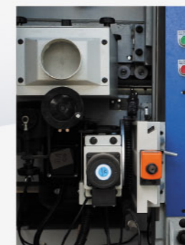
Disc sanding unit Motor : 2HP ,Spindle : 1"x 4" with vibration motor with auto. compensation
