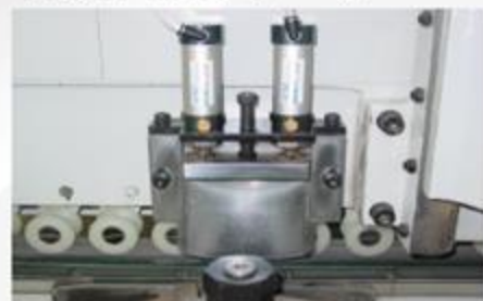
立轴加装气压式上下导板 Moulding unit with pneumatic top pressure pad+bottom support (Chrom plated)
