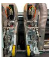
Left and right side shaping aggregate carrier with two HSK63 spindles each.
