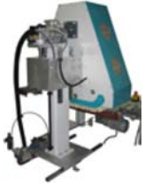
RB300 aggregate with motorized height setting and oscillation
